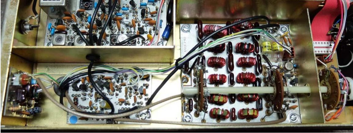
Figure 5 – Low Pass Filter Boards with no Cover
