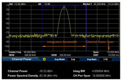
Figure 2-14 Channel Power Measurement Interface
