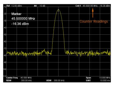
Figure 2-24 Frequency Counter Measurement
