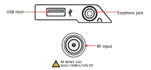
Figure 1-7 Front Panel Connectors
