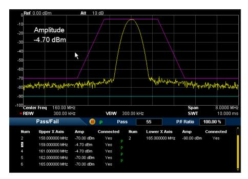
Figure 2-11 Interface of Pass/Fail Test
