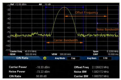
Figure 2-17 C/N Ratio Measurement Interface
