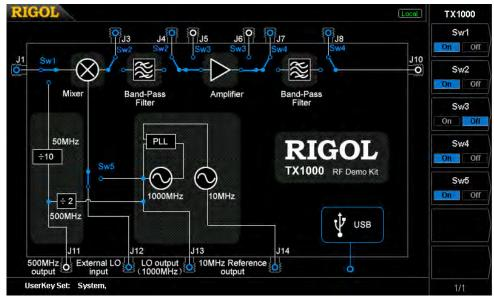
Figure 2-29 TX1000 control panel
