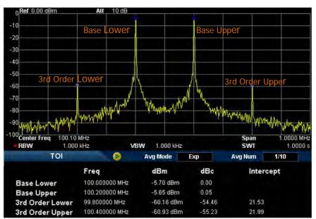
Figure 2-19 TOI Measurement Interface
