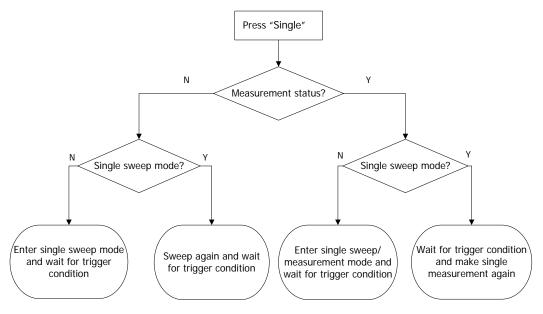
Figure 2-10 Process of Single Sweep
