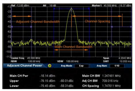
Figure 2-13 Adjacent Channel Power Measurement Interface
