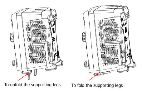
Figure 1-3 To Adjust the Supporting Legs
