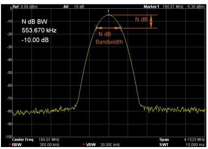
Figure 2-23 N dB BW measurement
