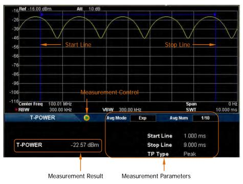
Figure 2-12 T-Power Measurement Interface
