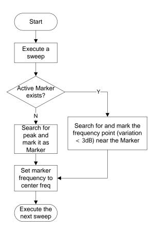
Figure 2-1 Process of Signal Track
