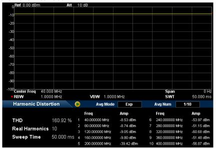
Figure 2-18 Harmonic Distortion Measurement Interface
