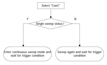
Figure 2-9 Process of Continuous Sweep
