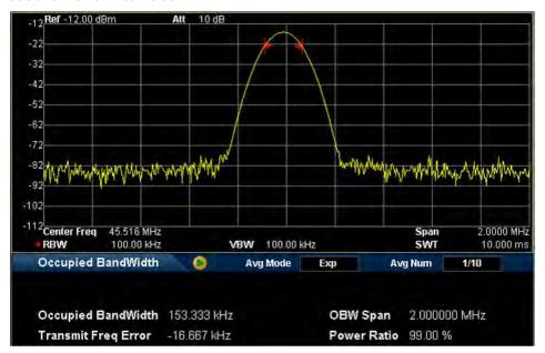
Figure 2-15 OBW Measurement Interface
