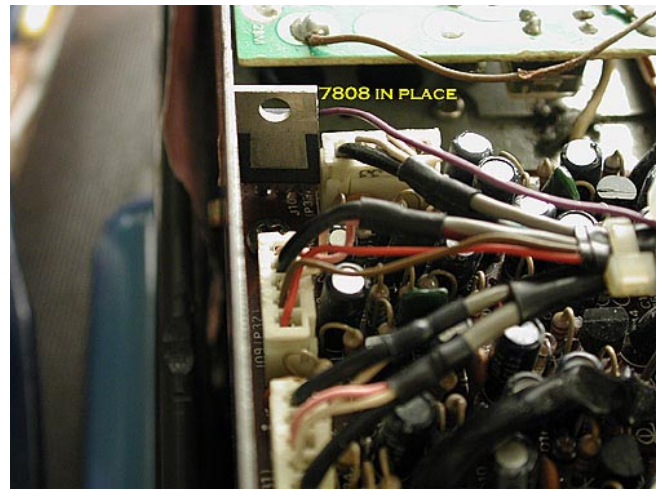
Figure 11 - Reinstall the AF and AM/FM boards and test. Again note the orientation of the 7808 at the time of final installation in the photo. The plastic part with writing should face toward the PA board.
