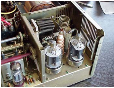
The PA with 6146A and 6146B tube
